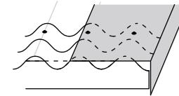
Alternatively, you could use one corrugation strip, cut from an ONDURA® Premium panel and place it under the last corrugation on the rake; or secure the last corrugation directly to a raised rake edge.
