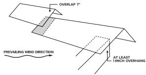
Insert closure strip between the panel and the ridge cap after all panels have been installed. The center of the closure strip should be 1 inch above the lowest end of the ridge cap. Close the area under the ridge at each end with a cap.
