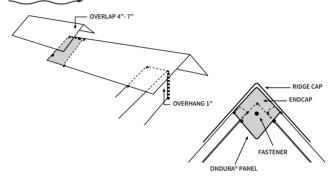
Insert ridge closure strip on the ONDURA® panel and under the ridge cap after all ONDURA® panels have been placed.
