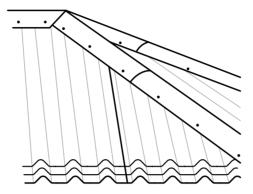
Snap chalk lines on each side of the hip to mark the area of the hip cover. See diagrams.
