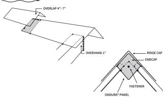
Insert ridge closure strip on the ONDURA® panel and under the ridge cap after all ONDURA® panels have been placed.
