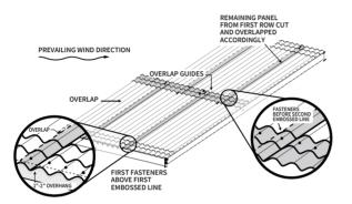
Each row should be installed with the first panel at the opposite end of the roof from the prevailing winds. With this orientation, the seam of the overlap will face away from the prevailing winds. If wind-driven rain could come from both directions, then we recommend sealing along the overlap with an elastomeric caulk.
