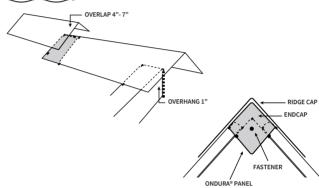
Insert ridge closure strip on the ONDURA® panel and under the ridge cap after all ONDURA® panels have been placed.
